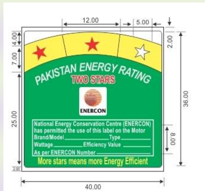
Figure-3: Dimensions of the Energy Efficiency Rating Label (all values in mm)
